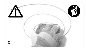
Hold the fan housing as shown in Fig. D and strike against a suitable surface (e.g. old newspapers - the spring is greasy!).
